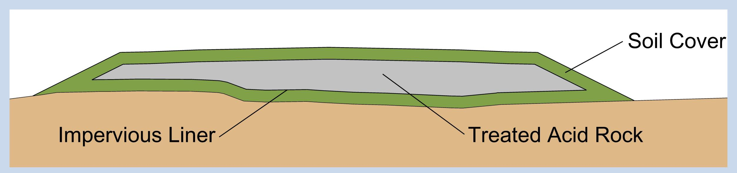
Typical section of treated acid rock with impervious liner and encapsulated.
